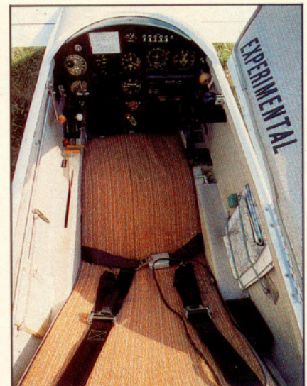
Modestly sized VariEze panel accommodates basic avionics and day-VFR instrumentation.
