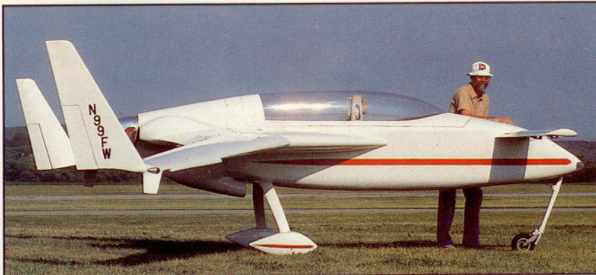
Fred Wimberly steadies his VariEze. The cockpit compares in size to the Long-EZ's, but VariEze wings have more sweep, less span and smaller fuel tanks and winglets.
