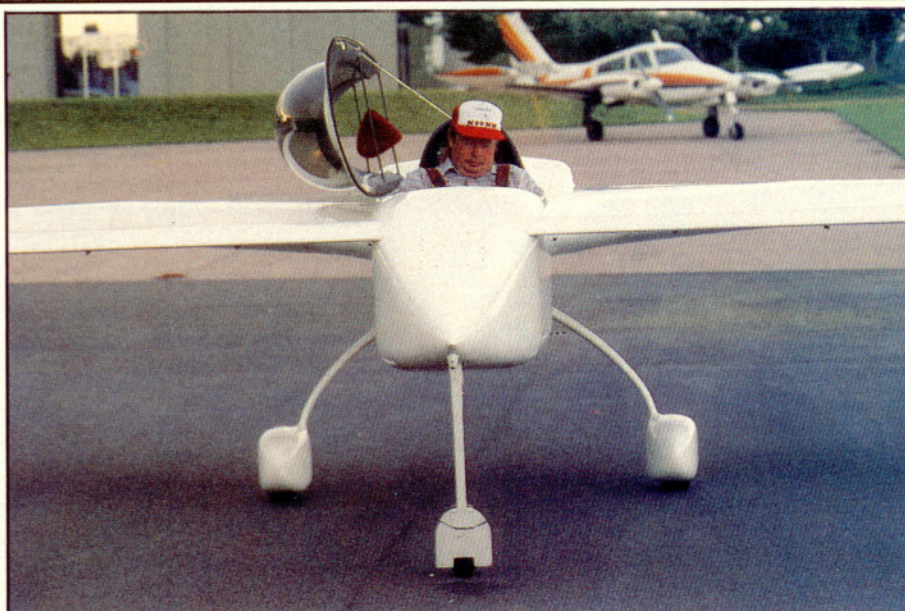
Red Morris dons his Long-EZ and prepares to lower the flip-top canopy. High speed on low power is possible because of the low frontal area of the tandem-seat fuselage, smaller wetted area of the tail-less design and smooth, rivet-free fiberglass surfaces.
