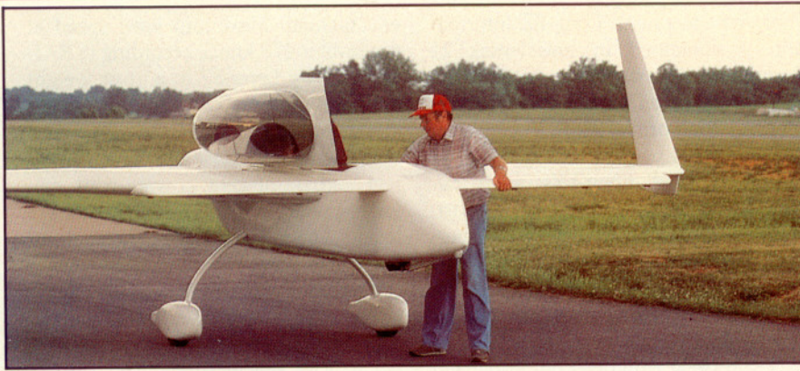
Morris wraps an arm around the canard of his Long-EZ to lift the snout and crank the nosewheel down. A small rubber disk protects the nose from scuffing when the EZ is grazing.
